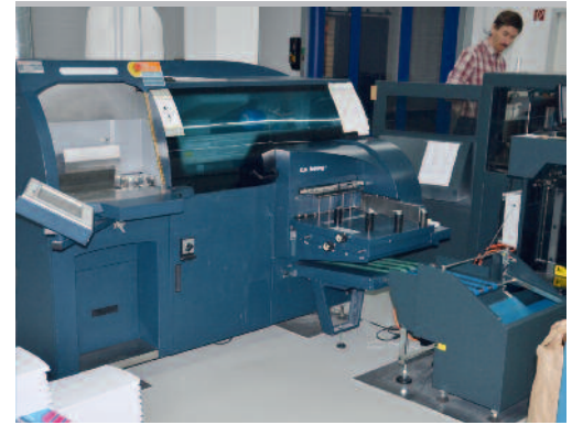
A C.P. Bourg perfect binding line handles the binding and trimming of the book blocks.
