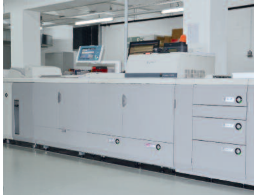
KN Digital Printforce uses a Canon Imagepress 6010 VP to print the colour title pages.
