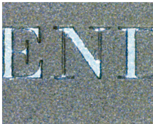
Figure 1: Distorted transfer of fine elements in the first batch.
